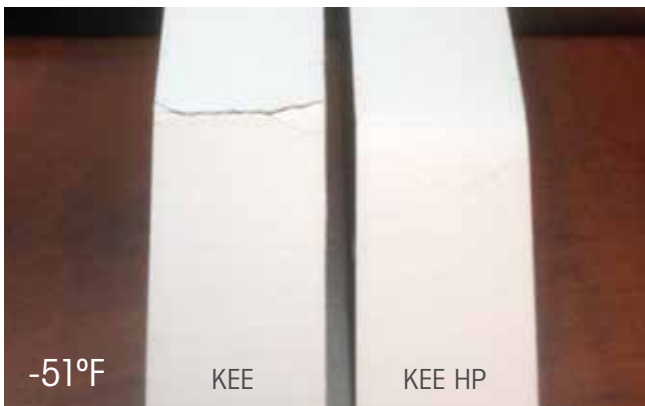
Same formulation except for the upgrade from standard KEE to KEE HP
